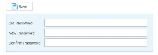
• To turn on Two Steps Authentication tick the box and click Save. This feature means that after entering your password, you will also be required to enter a code sent to your email address prior to being able to access the system. A greyed out ticked box means that your Supervisor has already set Two Steps Authentication:
